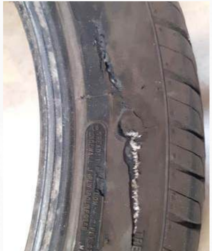
Fig 6. Damaged side wall caused by spring failure.
