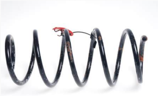
Fig 3. Surface defects on a spring after 1000 hours of salt spray testing
